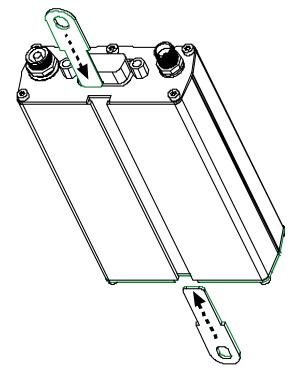
4. Attach the MultiModem with two screws to the mounting surface at the desired location on the equipment.
